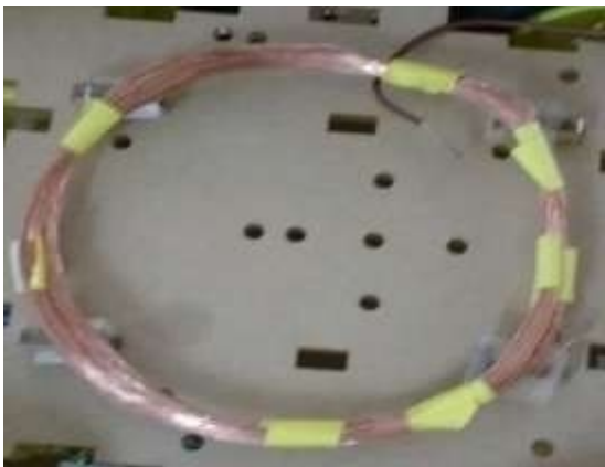
Fig. 4 Secondary coil designed for miniature model of Electric Car
