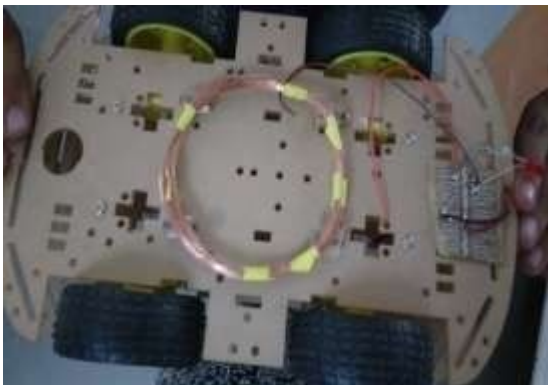
Fig. 5 Secondary coil mounted on miniature model of Electric Car
