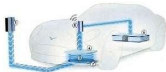
1-Power supply, 2-Primary coil, 3-wireless power Transfer, 4-Secondary coil, 5- system controller, 6-EV battery.
