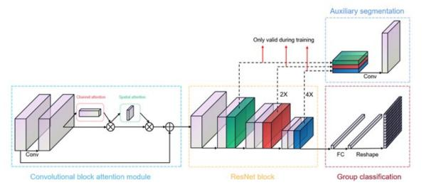
Fig. 2. Overall architecture with CBAM attention module.
