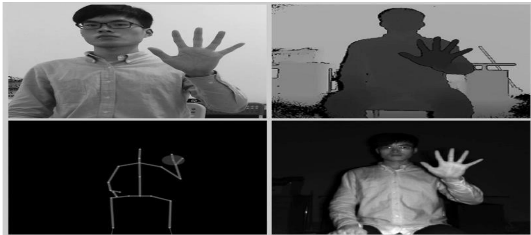
Fig.6. From left to right and top to bottom, there are a color image, a depth image, a skeleton image and an infrared image.
