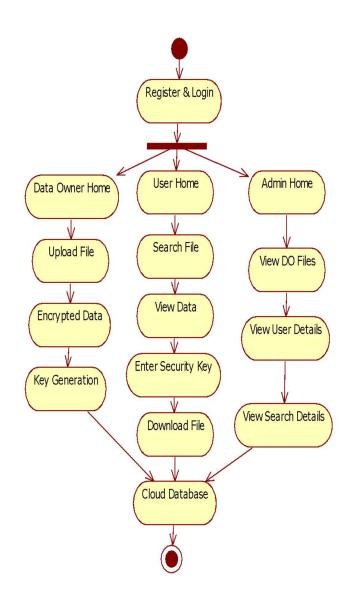
Activity diagrams are graphical representations of workflows of stepwise activities and actions with support for choice, iteration and concurrency. In the Unified Modeling Language, activity diagrams can **System Architecture**  be used to describe the business and operational step-by-step workflows of components in a system. An activity diagram shows the overall flow of control.
