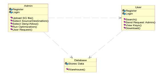
This class diagram represents how the classes with attributes and methods are linked together to perform the verification
