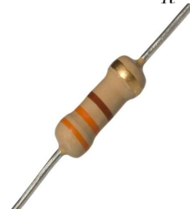
Fig 3.3.12: Resistor Bands In Resistor
