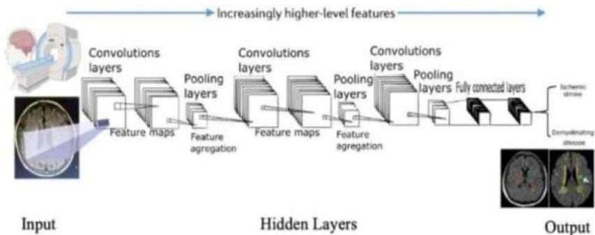
The model was trained using the Categorical Cross-Entropy loss function, optimized using the Adam optimizer with a learning rate of 0.001. Training was performed over 50 epochs, with early stopping employed to halt training when validation loss plateaued, thus preserving generalization capability.
