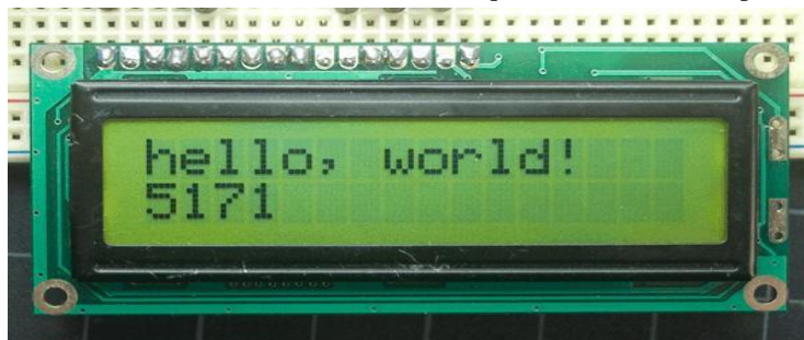
Output of the sketch on a 16x2 LCD
