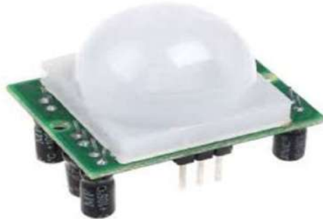
Fig.2. Passive Infrared Sensor [17]
