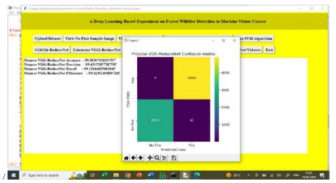
In above screen we are defining VGG16 as based classifier and then forming new model called VGG-REDUCENET by adding layers to extract Temporal and spatial features and In above screen with propose VGGREDUCENET we got 99.35% accuracy and we can see other metrics also
