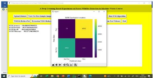
In above screen we are training SVM on train data and then evaluating its performance on test data and then SVM got 98% accuracy. In confusion matrix graph x-axis represents Predicted Labels and y-axis represents True Labels
