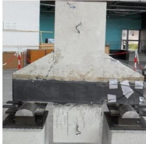
b) CB3u : Compression failure
