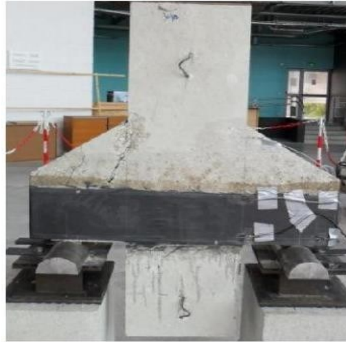
b) CB3u : Compression failure
