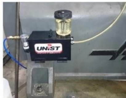
Fig 1: a) MQL supply with cryogenic
