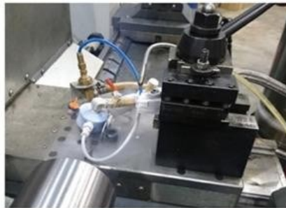
Fig 1: a) MQL supply with cryogenic
