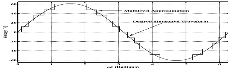
Fig.2 switching angle of multilevel inverter
