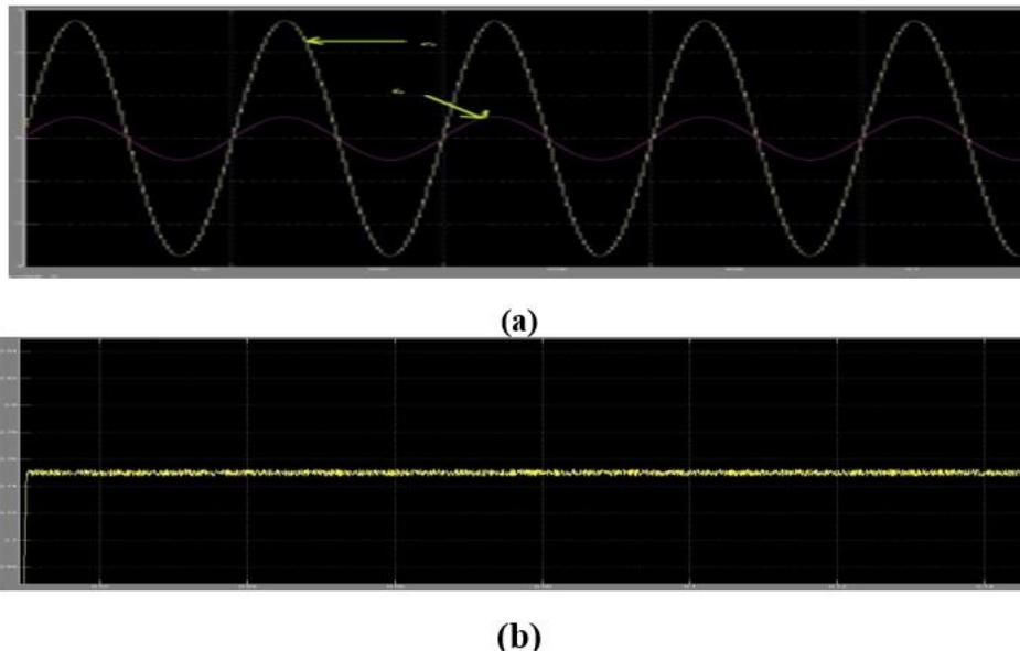
Fig 2. shows the waveforms of steady state three phase motor: (a) voltage and current of the grid, (b) dc-link voltage,
