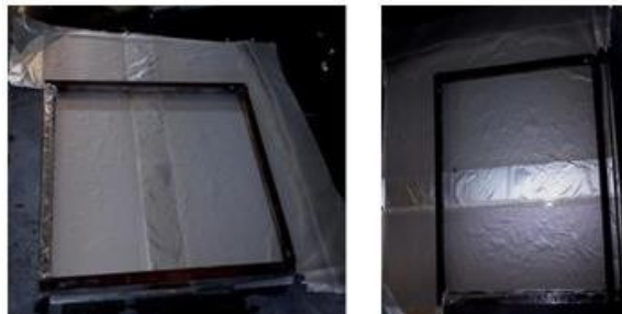
Figure 1: Aluminum foil is wrapped around the frame.
