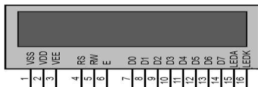
Fig 5: Schematic view of 16 x 2 LCD display
