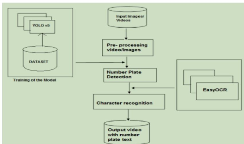
**YOLOv5 Model:** This component represents the training phase of the YOLOv5 object detection model.
