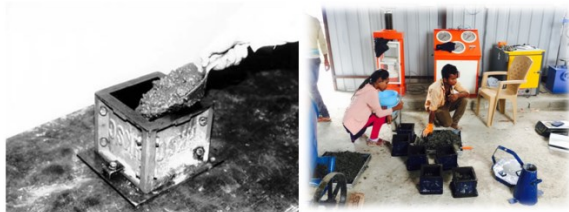
Filling the mould (for 150 mm cube 3 equal layers)
