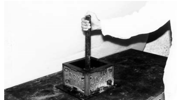
Compacting the concrete in the cube mould (For 150 mm cube at least 35 tamps per layer)
