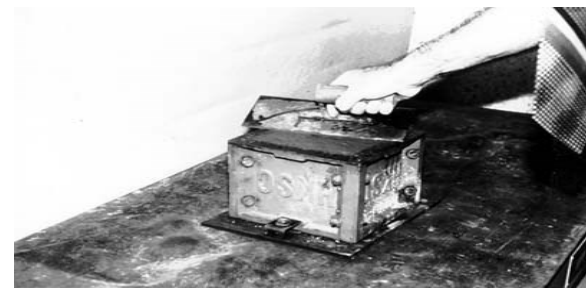
Compacting the concrete in the cube mould (For 150 mm cube at least 35 tamps per layer)
