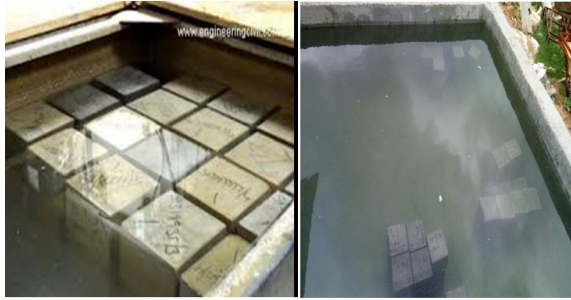
Curing of cubes and cylinders
